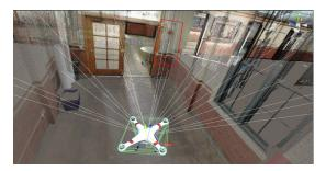
Figure 3. Digital drone equipped with laser for object detection (emergency exit lights and fire alarm panels)
