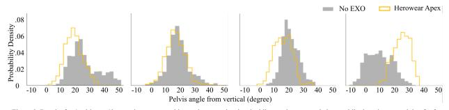
Figure 2. Results for 4 subjects. Changes in movement kinematics, unassisted and while wearing an exoskeleton while dumping a gondola of refuse into a larger cart.
